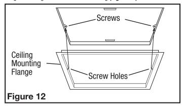
**NOTE:** If the housing is mounted to far or not far enough into the ceiling for the flange to make a solid connection, loosen the mounting channel and adjust the housing up or down on the rails. Once in place, fully tighten the mounting channel nuts.
