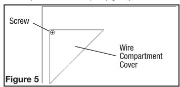
1b. Internal Wire Compartment: Using a 7/16" socket, remove the two hex nuts holding the blower assembly in place. Lift up on the assembly and slide it out of the tabs on the housing (Figure 6). Remove the wire compartment cover screw (or screws) and place the cover in a secure place (Figure 7).
